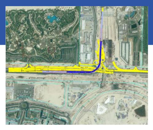
As part of Nakheel securing access to Jumeirah Gate Tower Project, Nakheel have retained Systra / AEC to study and design of the existing link to Palm Jumeirah Island from Al Sufouh Road. AEC were tasks to prepare the Concept Design as well as prepare the Detailed Design for Road and Utilities part of the project along with the related BOQ and Project Specifications.
