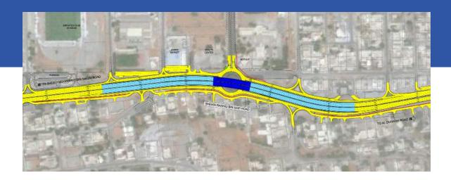
Ras Al Khaimah Palace Roundabout Improvement Project consists of increasing the number of travel lanes from two to three lane for each side of Sheikh Rashid Bin Said Road and upgrading the existing Palace Roundabout by introducing a new 3 span, 115m length, six lane bridge crossing the Roundabout to improve the traffic flow and enhance the traffic management of Al Dhait North and Al Dhait South.
