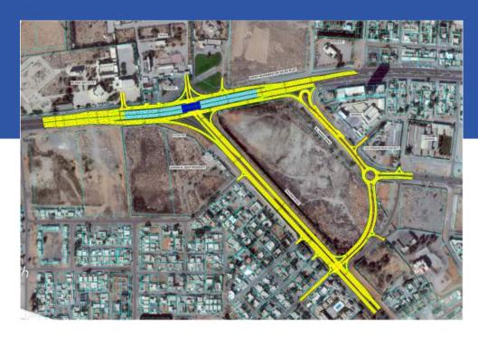
Ras Al Khaimah Clock Roundabout is located at the intersection between Sheikh Muhammad Bin Salem Road and Khuzam Road. The project consists of upgrading the existing intersection to cater the traffic flow, improve the traffic movements and enhance the traffic circulation. The improvement includes introducing 3 span, 115m long, six lane bridge along Sheikh Muhammad Bin Salem Road, widening Khuzam Road, installing new traffic signal and developing a new road connecting Khuzam Road and Nahda Road.
